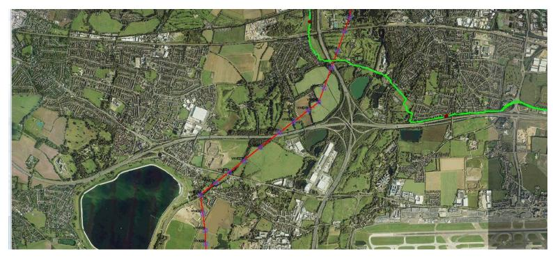
Red line = VW 275kV Overhead Line Iver – Laleham Iver – West Weybridge
